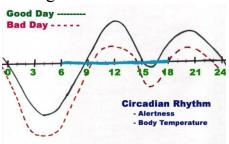
timeframe. It's been discovered that our inner core body temperature follows along this same line, but I've added Bad Day when you come to work already tired. Aloha's AMT's inspected those 1,300 rivets with the 140 cracks at exactly 3 to 5 am after having worked during the day before starting their midnight shift. The next article will describe the effects of that low.
